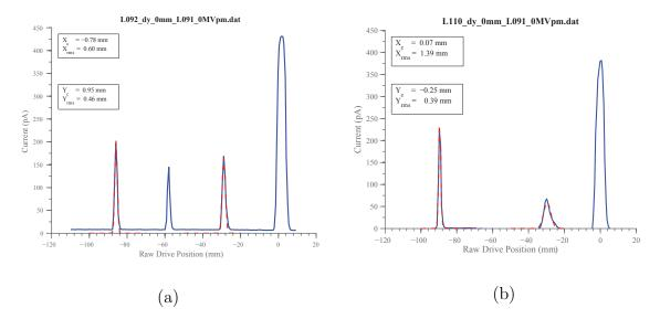
Figure 4.10: Plots of beam current vs. slit position for raw data from 45° slit scan taken at (a) L092 and (b) L110, and the Gaussian fit results for beam position and RMS beam size. Note that the 45° plate at L110 does not have the 45° slit, which accounts for the missing peak in (b).
