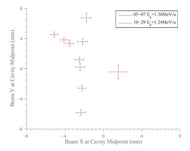
Figure 4.8: Beam position at cavity midpoint as projected from measurements at two downstream locations. Error bars are the RMS beam size. Note the improvement of the vertical separation and consistency of horizontal position achieved with the 10-29 data set which utilized the response matrix measurement technique.
