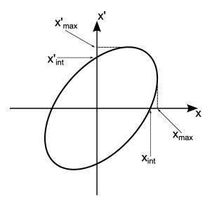
Figure 2.2: Phase space ellipse with negative  $\alpha$  (defocusing).
