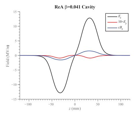
Figure 3.10: ReA  $\beta = 0.041$  Cavity Fields, including the accelerating electric field,  $E_z$ , and the transverse fields  $B_x$  and  $E_y$ . Note that  $E_y$  is very small, and so therefore has been multiplied by ten for the purposes of this graph.
