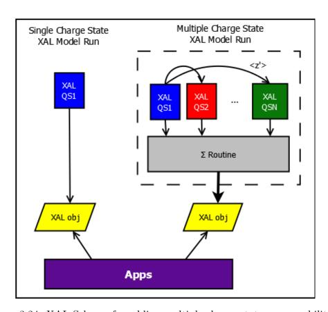
Figure 3.24: XAL Schema for adding multiple charge state run capabilities.
