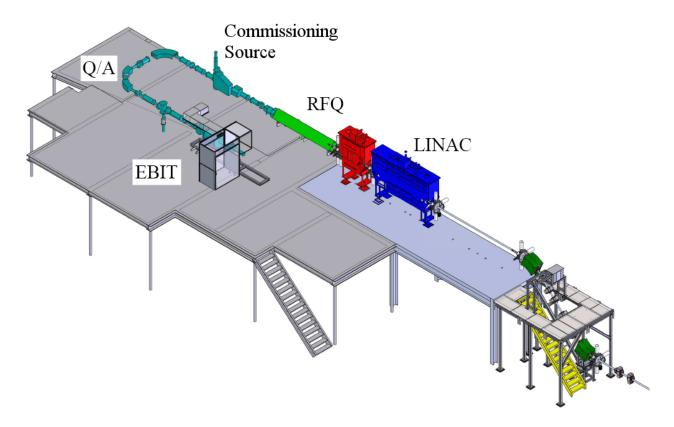
Figure 4.6: ReA Layout from 2013, including EBIT charge breeder, Q/A section, commissioning source, room temperature RFQ and superconducting linac including two cryomodules containing  $\beta=0.041$  accelerating cavities. Note the drift tube after the second cryomodule is the location for the third cryomodule containing  $\beta=0.085$  accelerating cavities, to be installed.
