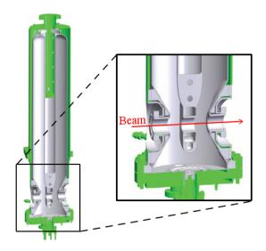
Figure 3.9: Cut-away image of the ReA  $\beta = 0.041$  QWR cavity type. The two accelerating gaps that the beam travels through towards the bottom of the cavity are shown in detail.
