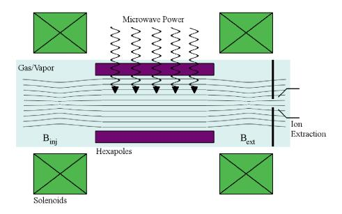
Figure 1.3: ECR schematic, including solenoid and hexapole coils. Microwave power,  $\omega_{RF}$ , creates the resonance zone in the center, and ion extraction is indicated to the right.
