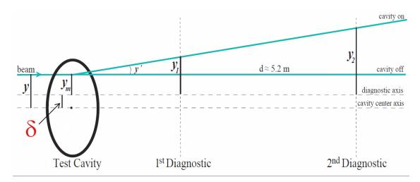
Figure 4.12: Schematic diagram of relevant measurement quantities depicting the difference between the diagnostic axis and the cavity center axis.
