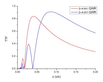
Figure 3.11: TTF of  $\beta = 0.041$  and  $\beta = 0.085$  cavities
