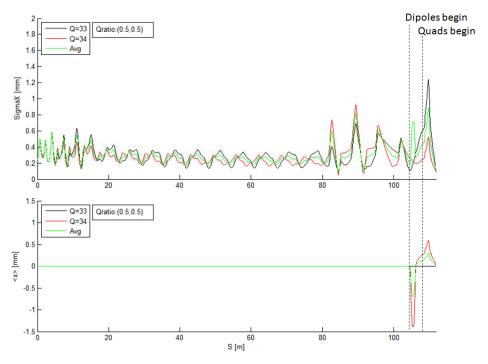
Figure 3.20: FRIB Linac Segment 1 as simulated by XAL for  $U^{33+}$  and  $U^{34+}$  charge states, as well as the result of the two charge states combined.
