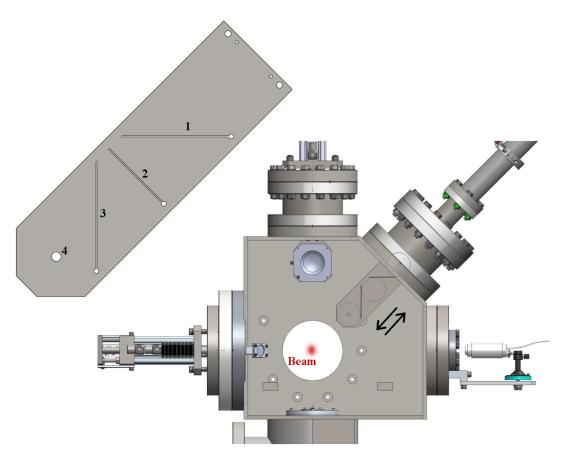
Figure 4.9:  $45^{\circ}$  Beam Profile Diagnostic setup. In the top left, the plate is shown with three slits and one aperture in the order that they intercept the beam during the profile scans: (1) the horizontal slit measuring the vertical beam profile, (2) the  $45^{\circ}$  slit for a measure of the coupling between the x and y planes, (3) the vertical slit measuring the horizontal beam profile, and (4) the 5 mm aperture for beam tuning.
