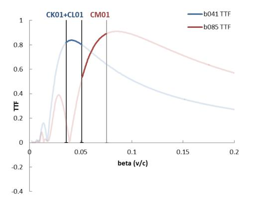
Figure 3.14: ReA TTF for  $\beta = 0.041$  and  $\beta = 0.085$  cavities, with operating regimes highlighted. The  $\beta = 0.041$  cavities are located in the first two cryomodules, CK01 and CL01, while the  $\beta = 0.085$  cavities are located in the third cyromodule, CM01.
