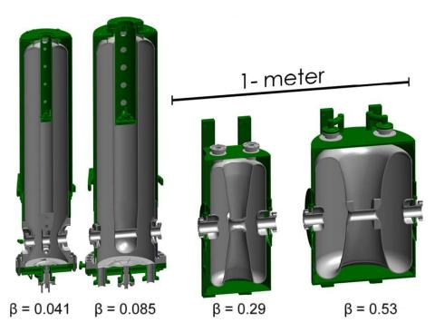
Figure 3.12: QWR and HWR Cavities [29]. The QWR cavities operate at 80.5 MHz, while the HWR cavities operate at 322 MHz.
