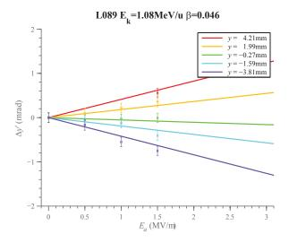
Figure A.2: Plot of  $\Delta y'$  vs.  $E_a$  for beam energies  $E_k = 1.08 \,\mathrm{MeV/u}$  ( $\beta = 0.046$ ). Lines correspond to the predicted response calculated using cavity design data and experimental conditions.
