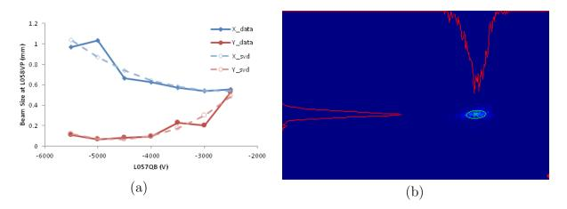
Figure 3.2: Left (a): Quad Scan Measurements performed before RFQ at ReA. Solid lines indicate measurement data, while dashed lines indicate SVD analysis. Right (b): Analyzed viewer data for L057QB=-5.5 kV with overlay of beam position and RMS beam size in green. Beam profiles in red are shown above and to the left of the beam spot.
