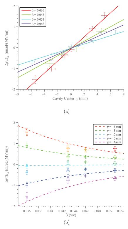
Figure 4.14: Left (a): Plot of  $\Delta y'/E_a$  vs. y at the midpoint of the test cavity, including each measurement data set. Note the agreement in the slopes for the different energies. Right (b): Plot of  $\Delta y'/E_a$  vs.  $\beta$  including each measurement data set.
