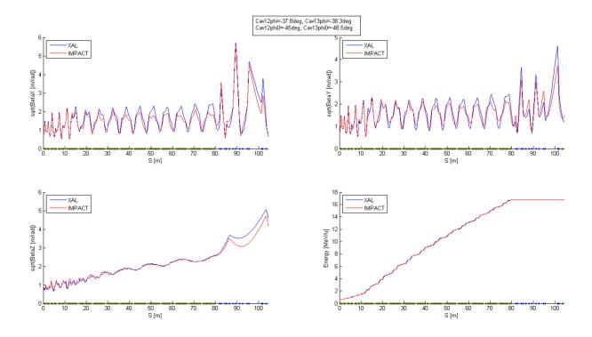
Figure 3.17: XAL Cavity Benchmark with IMPACT for a  $U^{33+}$  beam through FRIB's Linac Segment 1 to the Stripper Foil, including modeling of  $\beta = 0.041$  and  $\beta = 0.085$  cavities.
