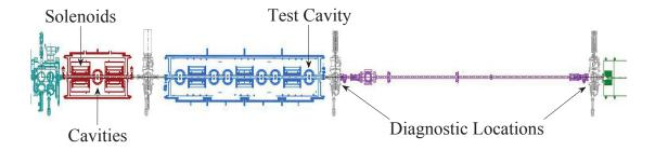
Figure 4.7: Schematic of ReA Linac as commissioned in 2013, before the installation of the third cryomodule. Square elements represent superconducting solenoids, while circular elements represent quarter-wave resonators. The drift space between the diagnostics after the second cryomodule is  $\sim 5.2 \,\mathrm{m}$ .
