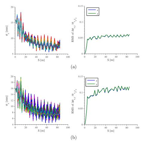
Figure 3.8: FRIB Linac Segment 1 (XAL) with random Gaussian error added to each solenoid. Gaussian errors of about (a)0.5% and (b)1% have been used — note how the RMS of the relative difference in  $\sigma_{x,y}$  grows by approximately the percentage of the Gaussian error introduced to the system. It is an important result that this growth levels out without increasing exponentially.
