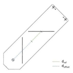
Figure 4.11:  $45^{\circ}$  Beam Profile Diagnostic Plate shown with distances from Equation 4.12,  $d_{\text{ref}}$  and  $d_{\text{offset}}$ , labeled.
