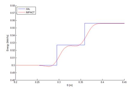
Figure 3.15: Modeling two gap acceleration in XAL as compared with IMPACT for a  $\beta = 0.041$  accelerating cavity.
