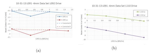
Figure A.1: Final measurement of L091 data set on 10-31. The  $E_a = 0.5 \,\mathrm{MV/m}$  L092 data point had all peaks shifted by the same amount. The dashed lines indicate where this overall shift has been manually accounted for in the analysis. L110 data indicates it was an issue with the L092 drive, not a sudden change in the beam, for instance from an instability in the LB source.
