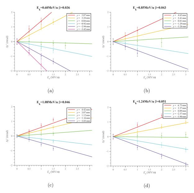
Figure 4.13: Plots of  $\Delta y'$  vs.  $E_a$  for beam energies (a)  $E_k = 0.6\,\mathrm{MeV/u}$  ( $\beta = 0.036$ ), (b)  $E_k = 0.85\,\mathrm{MeV/u}$  ( $\beta = 0.043$ ), (c)  $E_k = 1.08\,\mathrm{MeV/u}$  ( $\beta = 0.046$ ), and (d)  $E_k = 1.24\,\mathrm{MeV/u}$  ( $\beta = 0.051$ ). Lines correspond to the predicted response calculated using cavity design data and experimental conditions.
