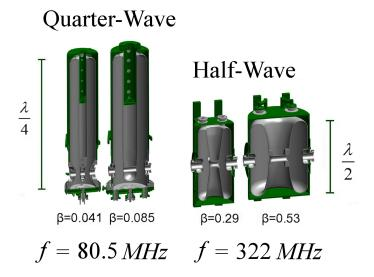
Figure 4.1: FRIB Quarter-Waver Resonator (QWR) and Half-Wave Resonator (HWR) cavity types shown with optimal  $\beta$  and operational frequencies. The FRIB HWRs are designed for four times the frequency of the QWRs, resulting in their length being about half as long.
