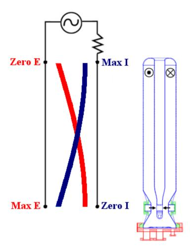
Figure 4.2: Coaxial Cable Analogy: the beam is accelerated at the open end of the "circuit" where the electric field is maximized, while the magnetic field circulates at the closed end.
