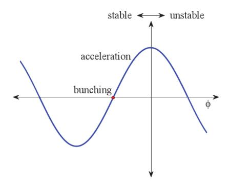
Figure 2.4: Longitudinal motion energy gain is proportional to  $\cos(\phi)$ . Points of zero energy gain (rebunching mode), stable acceleration (negative phase), and unstable region (positive phase) indicated.
