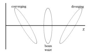
Figure 2.3: Phase space transformation of a converging beam along a drift space. After achieving a waist, the converging beam becomes diverging.
