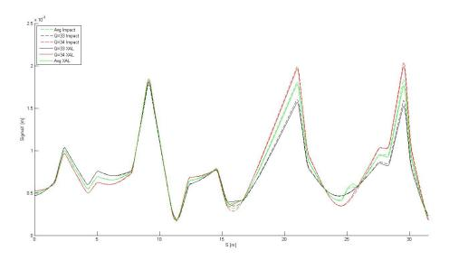
Figure 3.23: Results of XAL and IMPACT calculations for FRIB FS1 to Stripper. The IMPACT results are shown with dashed lines, while the XAL results are shown with the solid lines.
