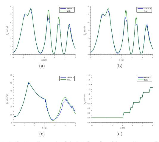
Figure 3.16: Benchmarking results of the ReA linac through its second cryomodule show good agreement between the matrix modeling code XAL, and the multi-particle tracking code IMPACT. Plots show the results for transverse  $\beta$  functions (a)  $\beta_x$  and (b)  $\beta_y$ , longitudinal  $\beta$  function (c)  $\beta_z$ , and finally the kinetic energy per nucleon, (d)  $E_k$ .
