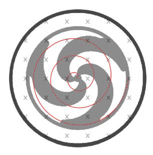
Figure 1.4: Cyclotron Schematic, depicting simplified beam path in red, alternating charge on "dees" with beam's relative position, and magnetic field into the page.
