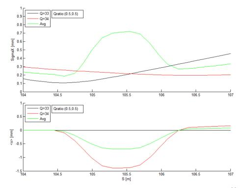
Figure 3.21: End of FRIB Linac Segment 1 chicane as simulated by XAL for  $U^{33+}$  and  $U^{34+}$  charge states, as well as the result of the two charge states combined.
