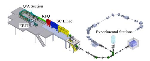
Figure 1.7: ReA layout including the accelerating linac on an elevated platform and the experimental stations on the ground level. The elevated deck design facilitates continuous access for laboratory personnel to other experimental areas.
