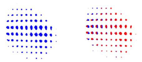
Figure 3.18: Results from ANL multiple charge state transport: pepper-pot image of the combined bismuth beam with charge states 20+ and 21+ (on the left) and superimposed images of  $^{209}Bi^{20+}$  (blue) and  $^{209}Bi^{21+}$  (red) beams transported individually (on the right) [51].
