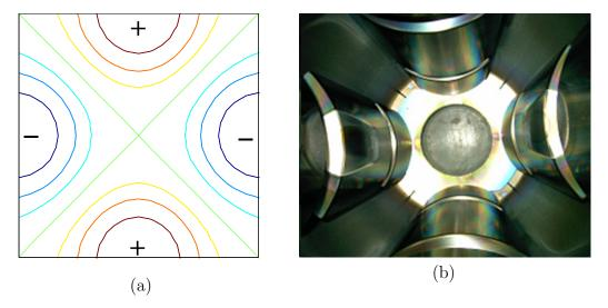
Figure 3.1: Left (a): Equipotential surfaces of quadrupole fields plotted for several different voltages. Right (b): The electrodes inside an actual electrostatic quadrupole are shaped along equipotential surfaces in order to produce a pure quadrupole field.
