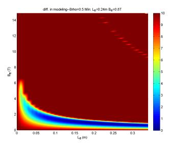
Figure 3.4: The ReA solenoid L090SN scaled to 1T for  $B\rho = 0.5\,\mathrm{T}$  m. The solution that minimized  $M_{\mathrm{tot}}$  is found to be at  $L_e = 0.24\,\mathrm{m}$ ,  $B_e = 0.8\,\mathrm{T}$ .
