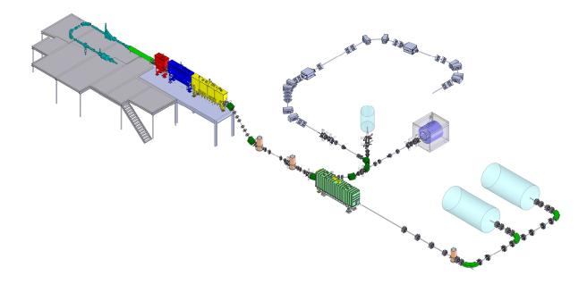
Figure 1.8: Planned layout for Energy Upgrade Phase I: ReA6. Note that additional single-cavity cryomodules have been added downstream from the original linac for longitudinal bunching, as well as an additional  $\beta = 0.085$  cryomodule for further acceleration. New experimental detectors will also be commissioned with the construction of ReA6.
