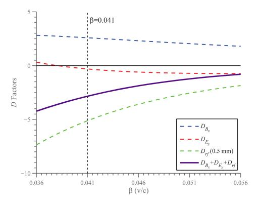
Figure 4.3: The calculated ReA  $\beta = 0.041$  cavity *D*-factors from Equation 4.6,  $D_{Bx}$ ,  $D_{Ey}$ , and  $D_{rf}$ , with  $E_a = 16 \,\mathrm{MV/m}$  and  $\phi = -90^{\circ}$  along with the sum of the three terms.
