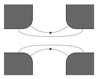
Figure 3.13: Electric field lines in an RF gap.
