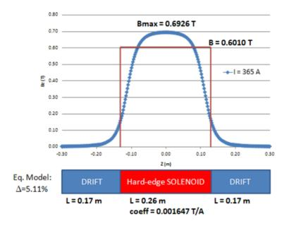
Figure 3.3: Equivalent hard-edge model for LEBT 0.6 T solenoid located before RFQ. The measured longitudinal field profile is shown with  $B_{\text{max}} = 0.6926 \,\text{T}$ , while the equivalent hard-edge model consists of a drift section ( $B = 0 \,\text{T}$ ), a constant field section ( $B = 0.6010 \,\text{T}$ ), followed by a second drift section ( $B = 0 \,\text{T}$ ).
