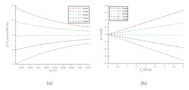
Figure 4.5: Left (a): Plot of ReA  $\beta = 0.041$  calculation  $\Delta y'$  vs.  $\beta$  for offsets dy = -6, -3, 0, 3, and 6 mm. Right (b):  $\Delta y'$  vs. cavity amplitude  $E_a$  for offsets dy = -6, -3, 0, 3, and 6 mm for beam energy  $E_k = 0.6 \,\text{MeV/u}$ , corresponding to  $\beta = 0.036$ .
