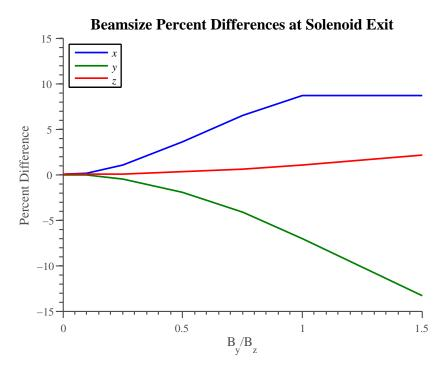
Figure 3.7: Percent difference between the "full-field" and "thin-lens" models for beamsizes calculated at the solenoid exit,  $z = 0.2 \,\mathrm{m}$ , as a function of relative corrector field strength,  $B_y$ , to the main solenoid field,  $B_z = 2 \,\mathrm{T}$ .
