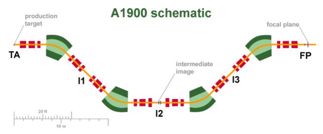
Figure 1.6: A1900 schematic, including four dipole magnets with maximum magnetic rigidity of 6 Tm. Production target, intermediate image, and focal plane locations also indicated.
